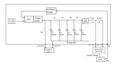
The APLL simulation tool models the NS3D02's analog loop filter as a 2nd-order passive loop. Unlike traditional PLLs where the full loop filter is external, the NS3D02 requires only a single external capacitor (C0).
